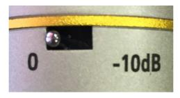
The "-10 dB" setting decreases the sensitivity with flat response, for example for outdoor or stage use, very close to the mouth of a speaker, singer, wind instrument, or any other situation where sound pressure can be excessive.
