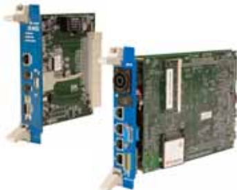
BC 2230 Master Controller Board w. 1 external Access USB, and Ethernet connectivity. Each System Chassis requires at least one controller. Two units may be installed in the same rack for redundancy purposes.
