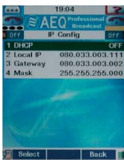
Manually configure IP parameters, or do it automatically with DHCP.
