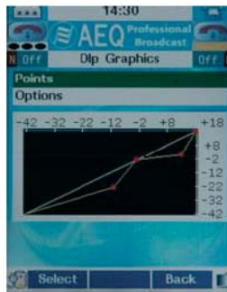
Fully configurable and graphical display of dynamics processing.
