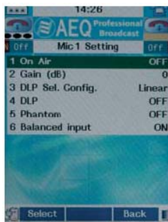
Fully configurable input parameters - DLP, Phantom feed, etc.
