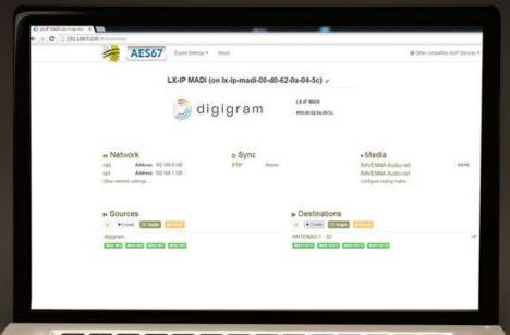
At this point we are already receiving the audio channels of the AES-67 stream generated from the BC 2000D. To leave doubts, if we can, enter the "Config Matrix Routing" window and select that the AoIP audio received by the ethernet interface RAO is routed to the outputs 1,2,3 4 of the MADI for its external check. It could be routed also to the analog outputs of the PC itself (dawo..daw3), but in this test for convenience we use the MADI interface that also has the card, to test the audio later.
