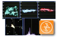
New tools have been included to assist in the signal monitoring, such as independent waveforms for Y, Cb and Cr, vectorscope and histogram, displayed in different colours for a quick identification of each tool.
