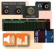
Audio monitoring is possible thanks to the different input options (analogue and SDI-embedded) and outputs (analogue, digital AES-EBU, headphones and stereo built-in speakers).
