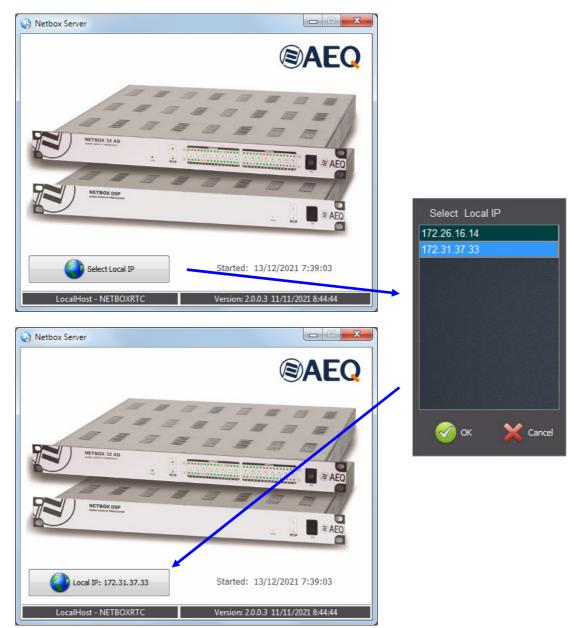
**Observation:** It's recommended that the database and "NetboxServer" are located on the same Computer. The .ini files of RTC and Server allows you to change some information as host, user, password or database.
