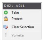
For each crosspoint you can "**Take**" (activate or deactivate) or "**Protect**" it and also see the physical connections (input connected to output). The "**Clear Selection**" option will clear any selection of crosspoints on the XY view.
