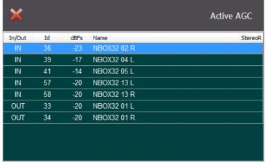
In the case of **NETBOX 32/8 AD MX** you can activate **AGCs only** in the input and output **Dante lines**, not in the analog or digital lines.
