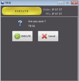
When the "Talkback" is executed all the existing crosspoints towards the output lines that are part of it will be deleted (towards the line defined as "PFL" as well as towards the ones defined as "Talk") and, only in the case of a NETBOX DSP, the gains of all the crosspoints (activated or not) towards those output lines will be restored to 0.
