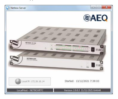
In the lower part of this window the IP address that will be used for the connection to NETBOX unit is shown (that IP address must be of the same range than the one for the unit). The date and time the application was started is also shown and, in the lower line, the database you're connected to and the application version (besides date and time of compilation) are shown.
