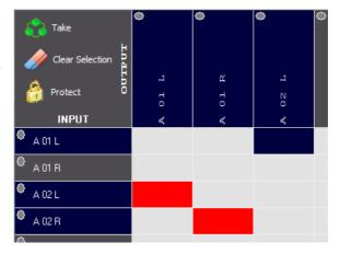
If a set of active and inactive crosspoints are selected (they will be marked in red and green respectively) and "Take" is executed, the "NetboxRTC" application will execute both the connections and disconnections, i.e. it's possible to both activate and deactivate multiple crosspoints with the same "Take" action.
