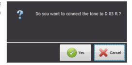
In case that this routing is already active, the option appears as "Tone OFF" and allows to deactivate it. Confirmation is also required.
