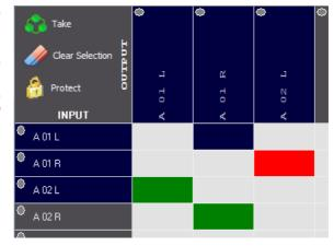
At the bottom of the window, the input and output associated with each crosspoint will be displayed when the mouse cursor is placed over that crosspoint.
