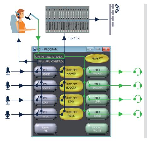
A "Talkback" group is a combination of input and output lines allowing for the automatic execution of an N-1 routing between these lines. In the default example, Madrid listens to Bogotá, Lima and Paris. Bogotá hears Madrid, Lima and Paris, and so on with the remaining two locations.
