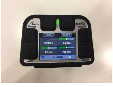
TV Sorocaba adquired in 2019 a CrossNET Intercom System. The system includes, among other elements, a CrossNET 72 matrix, 10 TP 8116 user panels, one TP 8416 user panel, and a wireless System Xplorer.
