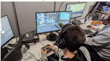
Finally for the commentators an AEQ OLYMPIA3 digital position is used, which is also connected via Dante to the matrix. The use of IP technology throughout the assembly simplified the wiring tasks, minimised the previous hours of installation, and allowed us to offer great versatility in the operation, with infinite changes in real time to adapt to a production as agile and dynamic as the live broadcasting of video game games requires.
