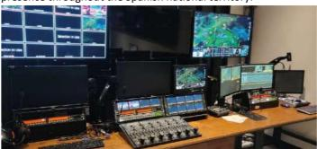
Secuoya has acquired for Riot Mexico, a leader company in Esports entertainment, a CrossNET 72 matrix for the main arena, 16 TP 8116 user panels, 9 Xplorer wireless belt packs with two multiple chargers and 4 WiFi access points. Two 6 to 1 concentrators were also supplied for communication with camera operators and intercommunication with audio consoles vía Dante and 4wired interfaces.
