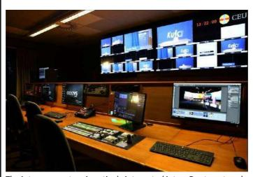
The intercom system is natively integrated into a Dante network that constitutes the audio backbone for both TV production and future audio and radio studios. This Dante network is integrated through a DANTE-MADI bridge with a hybrid broadcast video matrix with audio processing, so the intercom matrix also performs broadcast audio routing and distribution functions throughout the entire installation.
