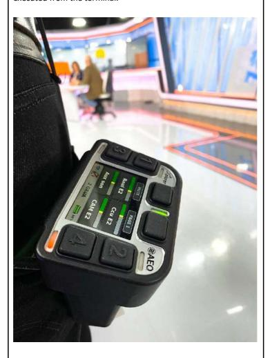
AEQ XPLORER is very comfortable for the user. Its dimensions and weight are reduced, protected from hits and splashes, it can be attached to a belt or hung from a strap, to use it as a shoulder strap. With autonomy for 20 hours of work, it can be recharged in a multiple base. It has a double assignable volume control, which can be configured, for example, to give direct access to the main speaker's level setting, differentiating it from the rest.
