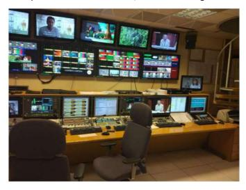
Thanks to the great flexibility of CONEXIA, the project implies a wide variety of panels in order to adjust to TV3's specific needs. TV3 system has 24 and 16-key user panels, with analogue, digital and even AoIP Dante audio.
