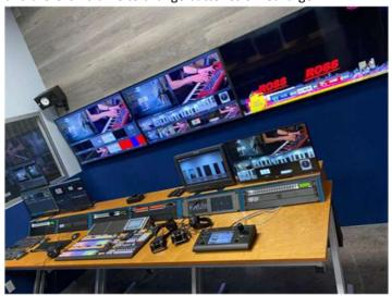
The entire system is integrated into the channels' AoIP flow and allows signals to be shared between the different contribution, intercom production and coordination systems. Specifically, the audio present in the AEQ Crossnet intercom matrix, coming from its ports and panels is also available on the Dante AoIP Network and any other equipment connected to it like for example the Allen & Heat SQ7 audio console, and could be broadcasted if so required.
