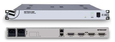
It can process up to 64 audio channels. Available processes include low-pass and high-pass filters, 4-band parametric equalizer, compressor, limiter, expander, noise gate and delay.
